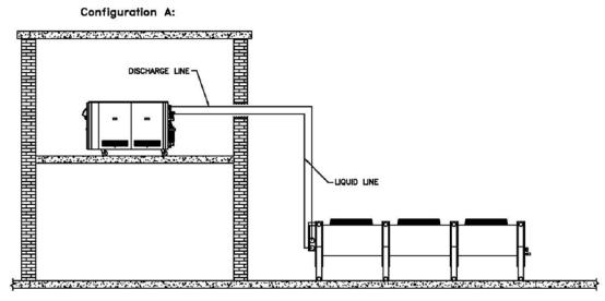
\* Liquid line riser should not exceed 15 feet from base of air-cooled condenser.
